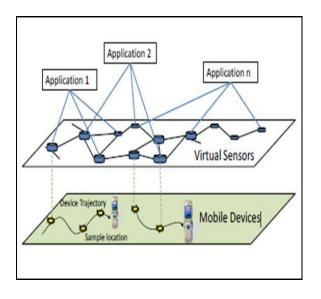
The virtual sensor nodes are supposed to hold the cache for the respective regions. The caches are updated based on requirement and is decided by the software.
